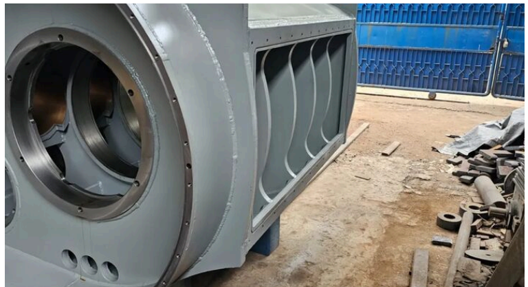
Welded internal ribs on a fabricated steel housing
