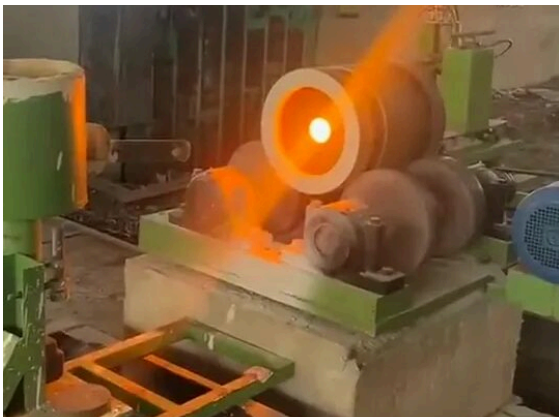
Centrifugal casting in progress
